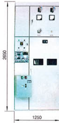
图 3 XGN2-12 旁路电缆出线柜外形结构图 Diagram 3 Outline structure of XGN2-12 bypass cable outgoing cabinet
